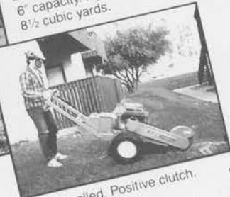
Full vision cutting. 22" wide. Hydrostatic drive.
