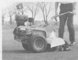
**Model "350"** . . . hand controlled, self-powered Turf-Quaker. Designed for greens and lawn maintenance . . . 23" wide, 6.2 H.P.
