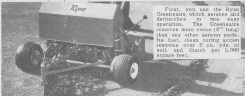
First, you use the Ryan Greensaire which aerates and dethatches in one easy operation. The Greensaire removes more cores (3" long) than any other aerator made. Its fast, clean coring action removes over 2 cu. yds. of soil and thatch per 5,000 square feet.
