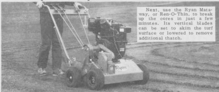
Next, use the Ryan Matabay, or Ren-O-Thin, to break up the cores in just a few minutes. Its vertical blades can be set to skim the turf surface or lowered to remove additional thatch.
