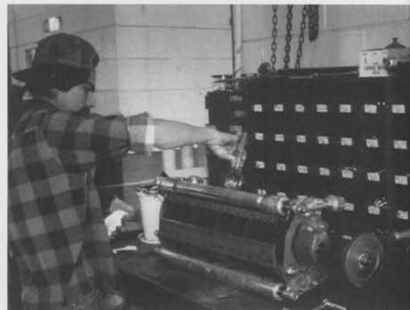
Reel maintenance is a very important part of turf equipment maintenance. Students learn how to grind, back lap and adjust reels.
