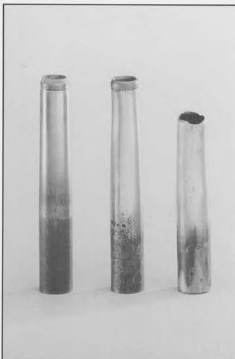
Left: an unused Dillennium Tine™ Center: a Dillennium Tine™ after 14 greens. Note the slight wall thinning, yet significant use-life still remains. Right: a conventional aerification tine used on the same course and machine at the same time after only 4 greens, completely worn out.
