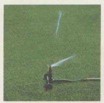
Avoid waste when watering slopes. A part-circle, impulse-type sprinkler, as shown here, provides slower delivery and gives better penetration. The flat, plastic, hose-type sprinkler is also good for this purpose, when fed with a reduced flow of water.
