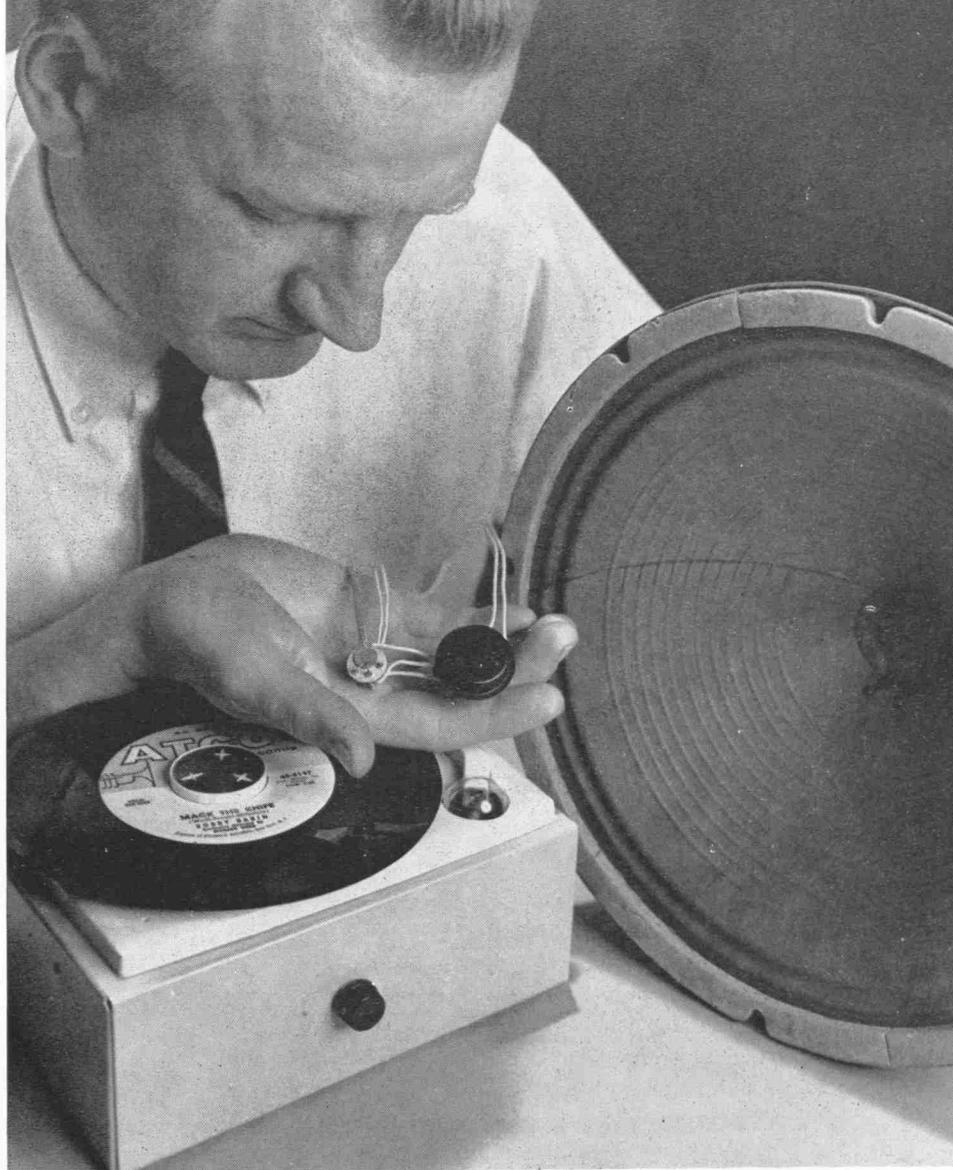
*A molecular electronic function block used as an amplifier in conjunction with a conventional preamplifier and speaker.*
