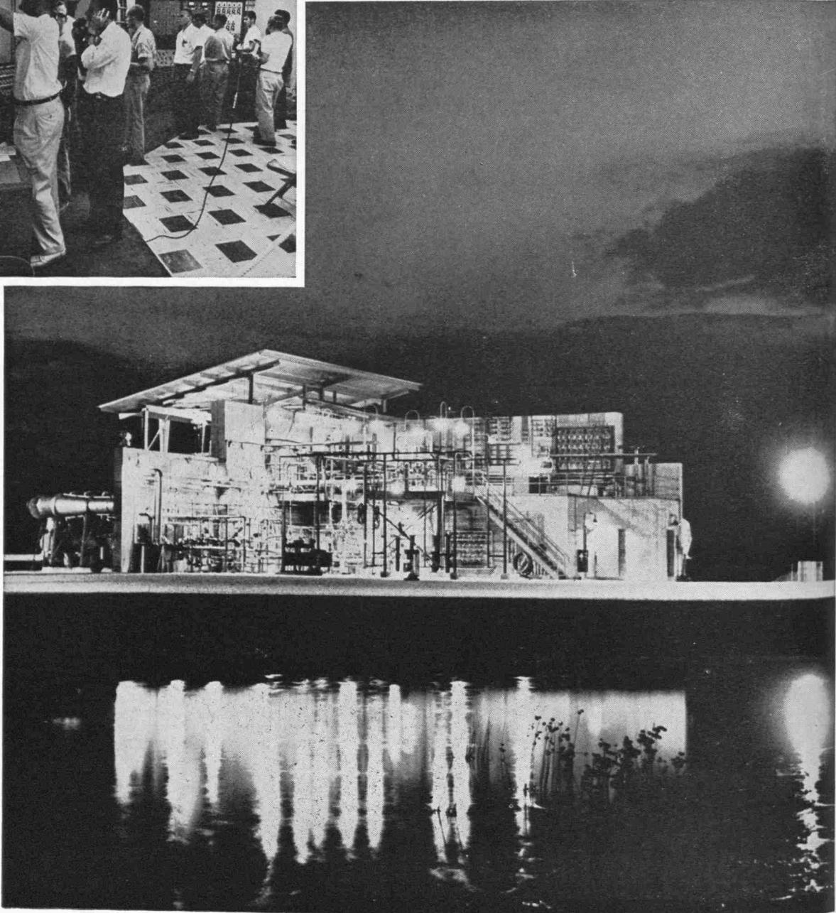
Development testing of liquid hydrogen-fueled rockets is carried out in specially built test stands like this at Pratt & Whitney Aircraft's Florida Research and Development Center. Every phase of an experimental engine test may be controlled by engineers from a remote blockhouse (inset), with closed-circuit television providing a means for visual observation.
