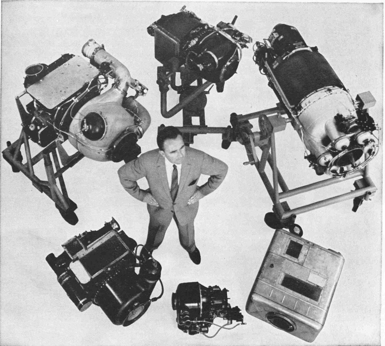
*Helmut Schelp, chief engineer, AiResearch Manufacturing Division of Arizona, Phoenix, surrounded by typical gas turbines now in production ranging in size from 30 to 850 hp. Clockwise from the top: GTC 85-28 GTC 105 • GTP 70-6 • GTP 30-1 • GTP 70-10 • GTU 85-2.*
