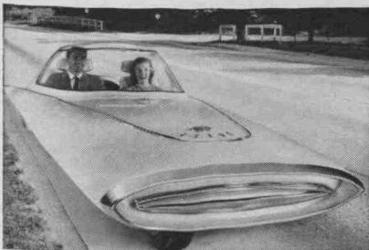
**Gyron**—dream car that drives itself. A gyroscope would stabilize this two-wheeled vehicle of the future, which envisions automatic speed and steering control. A computer would let you "program" trips on a non-stop highway. For lasting beauty, trim areas would be coated with Nickel-Chrome plating, the bright, corrosion-resistant finish.
