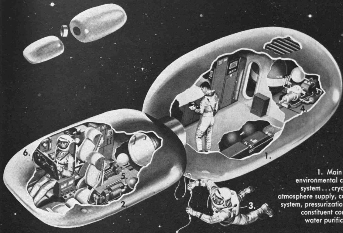
1. Main cabin environmental control system . . . cryogenic atmosphere supply, cooling system, pressurization and constituent controls, water purification.
