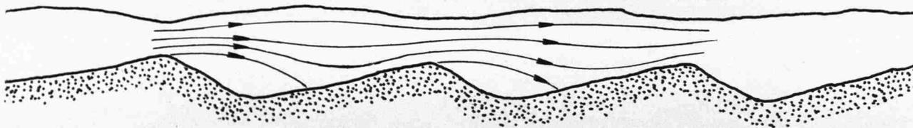
Fig. 1. Flow over a Dune Bed.
