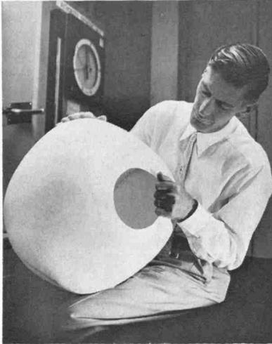
Once aloft and inflated, the object would soon rigidize and maintain its shape even though it was punctured by meteors, punished by temperature extremes, and exposed to ultraviolet radiation and other cosmic forces. These coatings are applied to the fabrics to impart a "rigidizing" capability and to form a film or barrier in the porous surface of the material so that it can be inflated when used in space structures.
