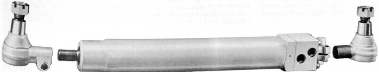
New power steering units mark Clark's entry into this mobile equipment field. They are designed for vehicles having axle load carrying capacities between 6,000 and 50,000 pounds.
