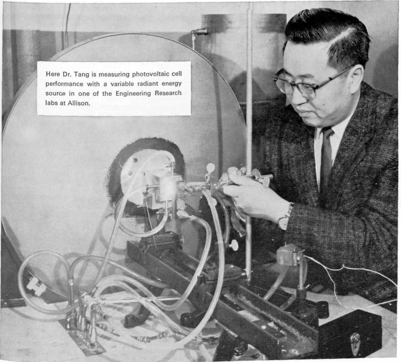
Here Dr. Tang is measuring photovoltaic cell performance with a variable radiant energy source in one of the Engineering Research labs at Allison.
