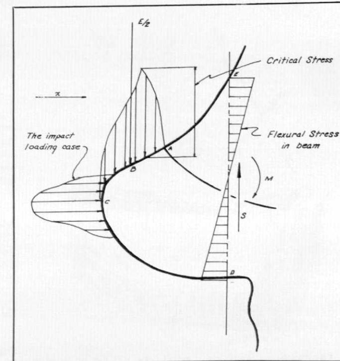
Fig. 2 at right is the bending moment diagram of the beam under shear stress and impact loading.
