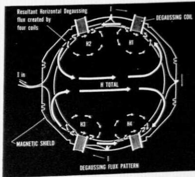
A voltage-dependent resistor, in series with the degaussing coils (wound on the picture tube shield), acts as a switch to connect the coils across the thermistor only during the warm-up of the receiver. Thus, the slow drawing away of the coil in manual degaussing is simulated automatically.
