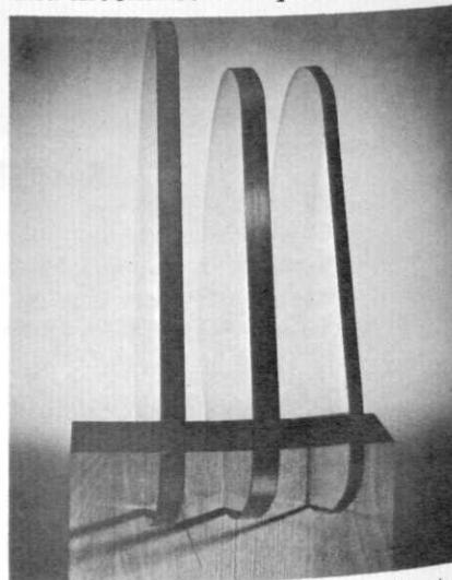
Edge-on view of panels of glass for the Gemini window illustrates relative thicknesses. Outer panel is at left; location of astronaut's eyes is at near-normal angle to the glass, at right.
