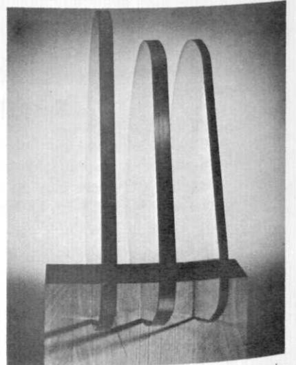
Edge-on view of panels of glass for the Gemini window illustrates relative thicknesses. Outer panel is at left; location of astronaut's eyes is at near-normal angle to the glass, at right.
