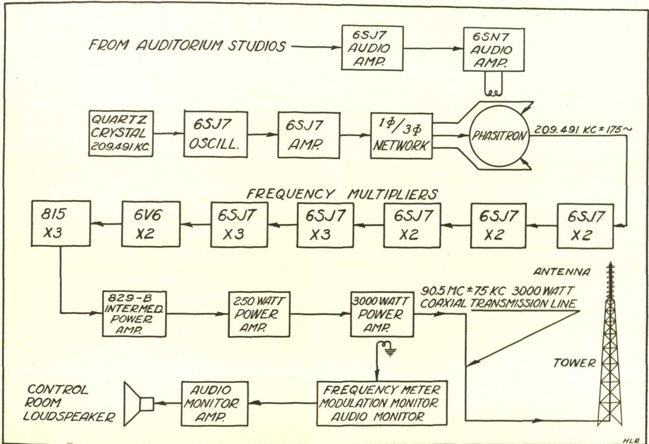
Fig. 1. Simplified Block Diagram
