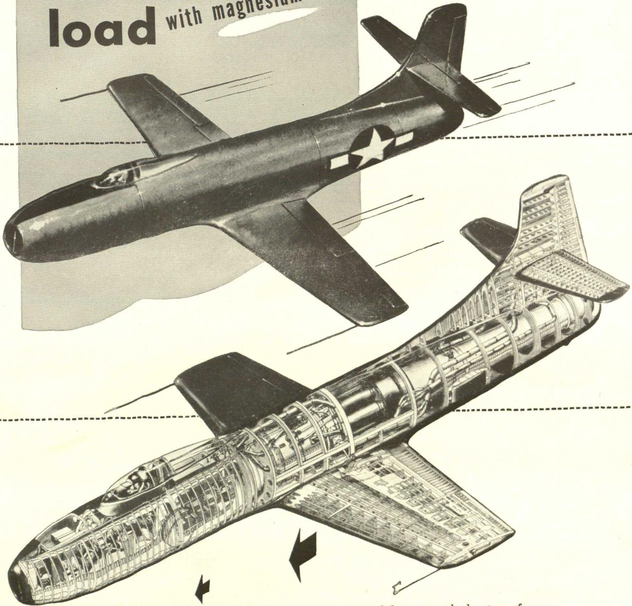
Here you see the Navy-Douglas D558 Skystreak—a dramatic demonstration of the structural advantage of magnesium. Strong magnesium alloy sheet is literally "wrapped" around the Skystreak's powerful jet engine to form the entire fuselage skin aft of the pilot seat. This makes possible a monocoque structure which completely eliminates the usual stringers, except for frames carrying concentrated loads.
