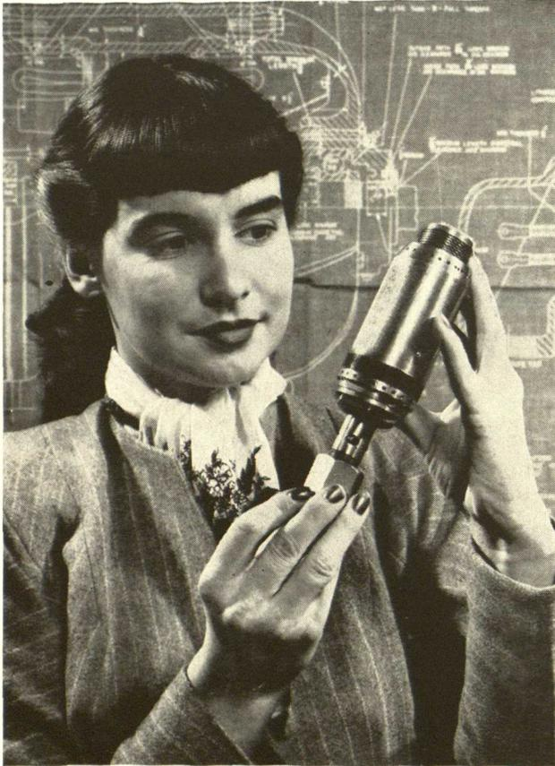
*This tiny electric motor is unusual in that it has been built "inside out." Developed for Army Ordnance's Proving Grounds, Aberdeen, Md., by the General Electric Company, it is rated one-tenth-horsepower at 80,000 revolutions per minute. The positions of the rotor and stator in the motor are the reverse of the usual arrangement, hence the term "inside out."*
