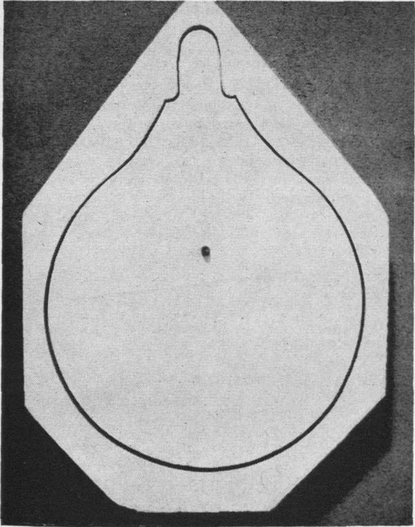
An original pattern and the expanded mold, made of high expansion cement. The neck shows that expansion is proportional. (U. S. Gypsum Co.)
