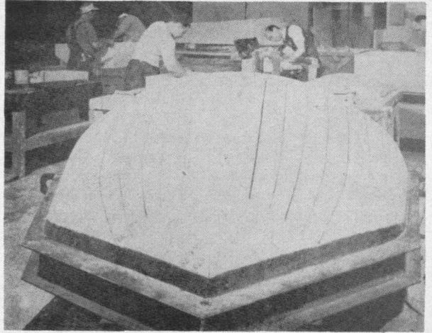
One of the many applications of gypsum cements. This is a master prototype model made by wiping the cement into a series of nested templates. (Douglas Aircraft Co.)
