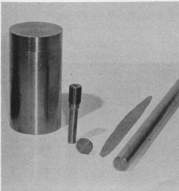
Several pieces of tooled titanium are shown above. Titanium may be used for high speed engine parts because of its high melting point (3150° F.)
