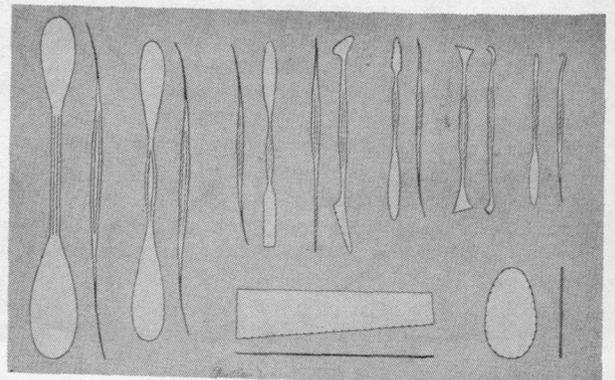
Some of the plasterer's tools include spatulas, scrapers, cutting and filing equipment, carving tools. (U. S. Gypsum Co.)
