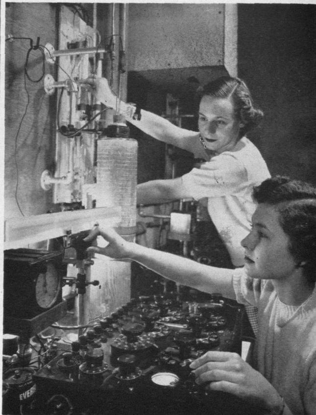
Determining the purity of a hydrocarbon by measuring its freezing point.
