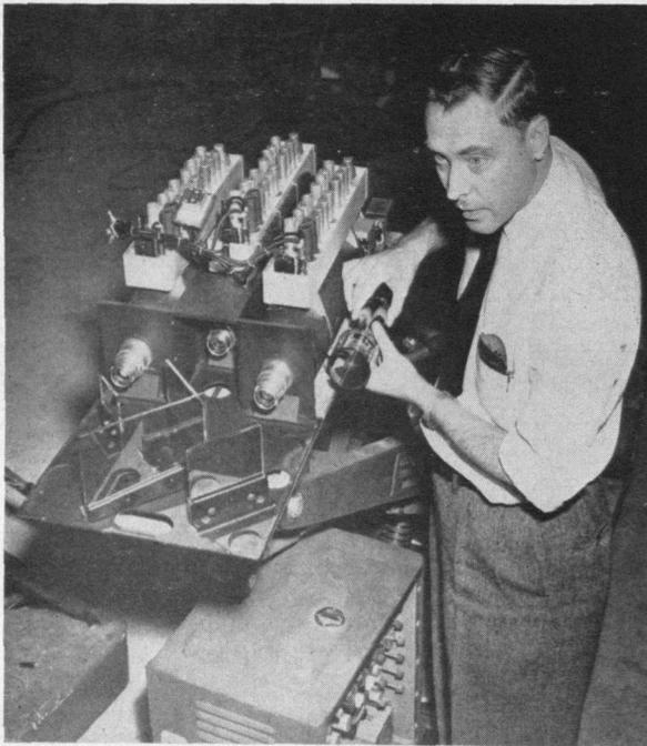
A view of the color camera showing the color separation setup. Each tube takes a one color image.
