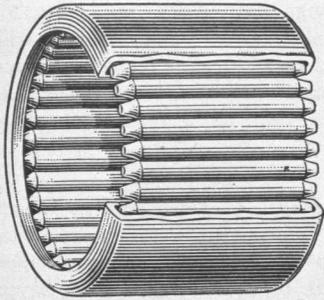
The Torrington Needle Bearing is a completely self-contained unit consisting of a full complement of small diameter rollers and a single retaining shell. This unit design and construction greatly simplify handling and speed assembly, and help reduce the size and weight of related parts.
