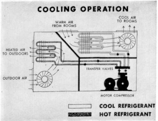
The Weathertron is compact in size and can pass through a 28-inch door. It can be placed in almost any location, garage, basement, alcove; any place that is convenient to the home owner. Since it does not burn any combustible fuel, its location is not dependent on a chimney, and in fact, the house does not need a chimney. The flexibility and function of the unit may have a profound influence on future home design.
