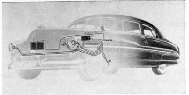
In its regular pattern of functioning, an oncoming car moving with its "brights" engaged, would cause the device to undergo a switching-action as soon as it appears on the device's horizon." Your headlights automatically go from bright to dim—stay that way until all oncoming traffic passes. When the opposite lane is clear they automatically return to bright.
