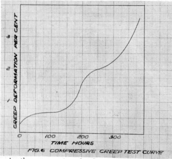
FIG. 6 COMPRESSIVE CREEP TEST CURVE
