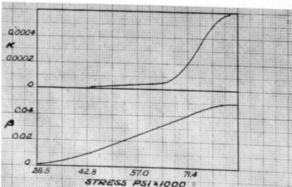
FIG. 3 VARIATION OF CONSTANTS K AND B WITH APPLIED STRESS FOR LEAD AT 60°F.
