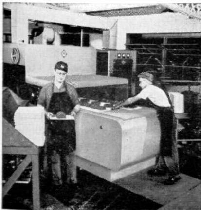
**ELECTRONICS**—Modern way to dry sand cores is with Allis-Chalmers *Foundromatic* Sand Core dryer. Revolutionary new process dries cores in minutes instead of hours.
