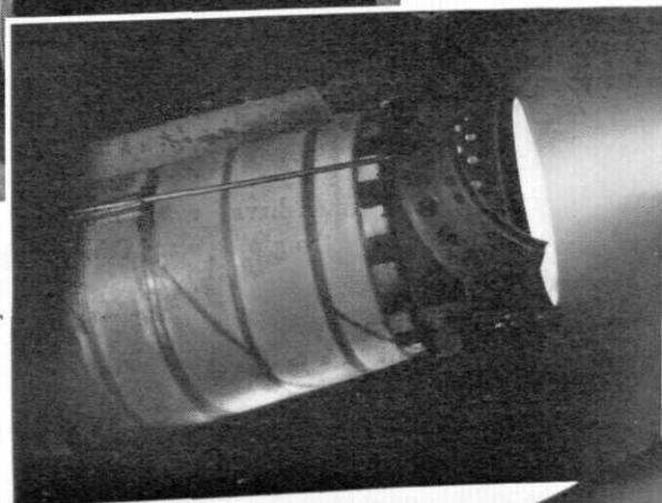
To stand up against intense heat and highly corrosive gases, vital jet engine parts such as rotor blades, afterburner, and insulation bindings are made of nickel alloys. Illustration shows a Pratt & Whitney Aircraft turbojet engine with afterburner.
