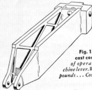
Fig. 1. Original cast construction of operating machine lever. Weighs 182 pounds . . . Costs \$38.25.
