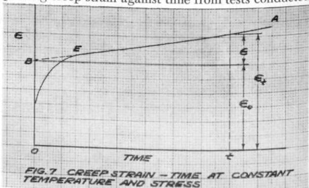
FIG. 7 CREEP STRAIN - TIME AT CONSTANT TEMPERATURE AND STRESS
