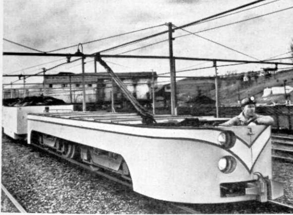
A modern high-speed, 30-ton mine locomotive hauls loaded coal cars from gathering tracks to coal tipples economically, quickly, and with a high degree of safety.
