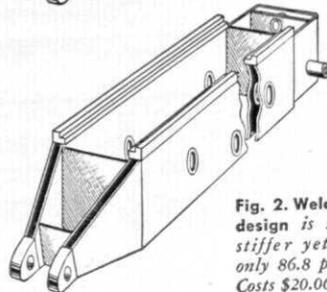
Fig. 2. Welded steel design is stronger, stiffer yet weighs only 86.8 pounds . . . Costs \$20.06.
