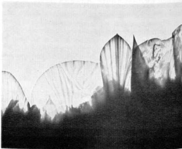
These delicate crystals may cause stress corrosion cracking.
