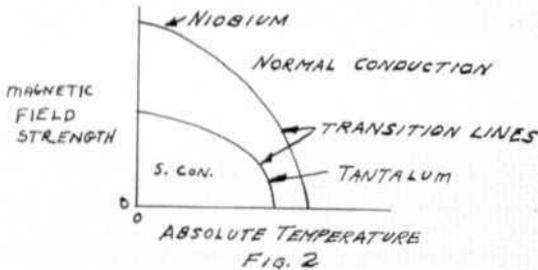
current to vary the resistance in the tantalum wire between superconduction and normal conduction, we can vary the amount of current flowing through it. With this arrangement we can then obtain current gain and power amplification, because a smaller current in the control winding will effect a larger current moving through the tantalum wire.
