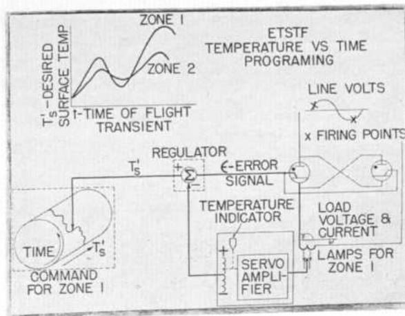
The second method considers the heat per unit time into the aircraft as proportional to the derivative of the skin temperature. A signal proportional to the power into the aircraft is obtained. The command signal, showing the power into the aircraft required to simulate a given flight trajectory, is developed by the computer. Using an injected coefficient of heat transfer and the effective temperature of compressed
