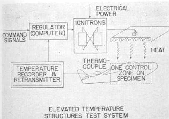
Sufficient gain is provided making the ignition unit applicable to other types of regulating controls which may be developed.
