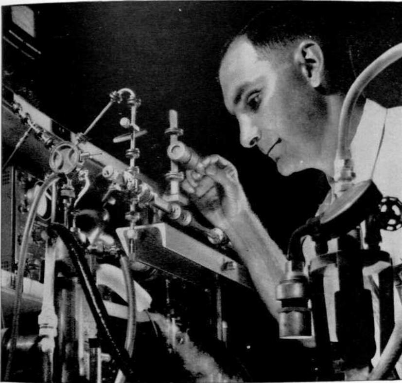
Dr. M. A. Biondi (Massachusetts Institute of Technology, B. S. '44, Ph. D. '49) measuring ultra-microwave transmission through superconductors. This experiment is a joint effort of a group of Westinghouse scientists aimed at obtaining a better understanding of the nature of superconductivity.
