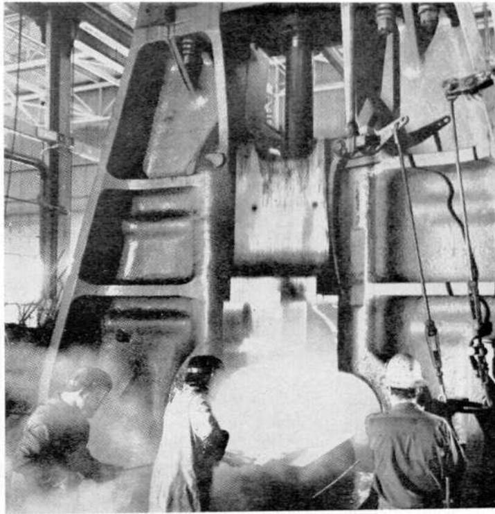
Grain flow of the metal undergoes a similar transformation, changing from a straight flow into an exact repetition of part contours.
