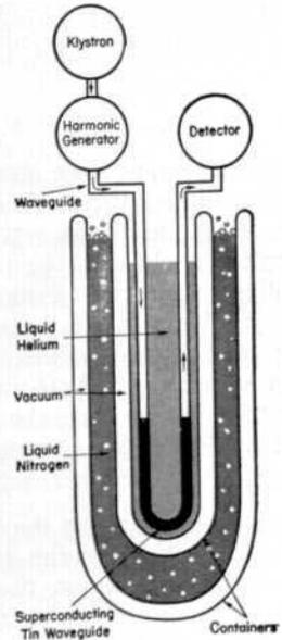
Highly simplified diagram of the apparatus used to study the absorption of millimeter wavelength microwaves in superconducting tin waveguide. Studies of this type have shown the existence of a gap in the energy levels of superconductors. These studies have thus provided key information in solving the puzzle of superconductivity.
