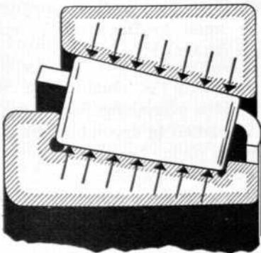
**How Timken bearings hold shafts rigid to maintain accuracy**—The full line contact between Timken bearing rollers and races gives shafts rigid support over a wide area. Shaft deflection is minimized. And the tapered design of Timken bearings permits them to be set up with the most desirable amount of end play or preload that gives the best performance.
