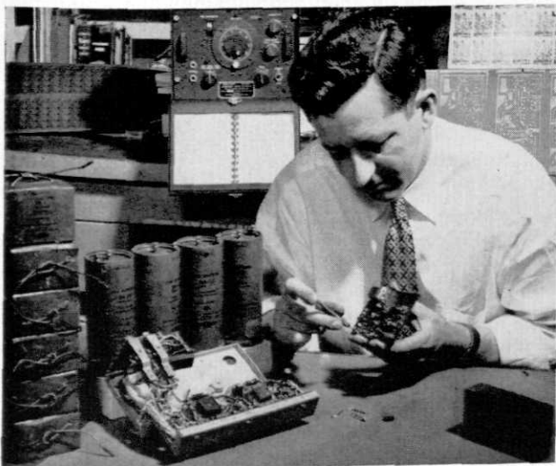
PRINTED CIRCUITS REDUCE SIZE: Signal Corps printed circuit techniques developed in the laboratories at Ft. Monmouth, have led to tremendous reductions in size and weight of military and commercial equipments. When used with transistors, a circuit for a frequency meter, as the one held by this scientist in his hand, plus small battery at right, replaces all the parts shown in conventional vacuum tube model pictured at left.
