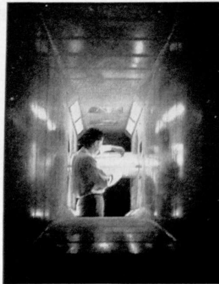
C. H. Fish, design engineer assigned to Lockheed's Icing Research Tunnel, measures impingement limits of ice on C-130 wing section. The tunnel has a temperature range of -40^{\circ}\text{F.} to +150^{\circ}\text{F.} and maximum speed of more than 270 mph. It is the only icing research tunnel in private industry.
