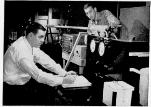
Mechanical Research Engineer W. M. Watkins (left) directs Research Mechanic Earl Rollo in operating Lockheed's new Hailstone Gun during a test on the effect of hailstones on new types of plastic radome "skin." The gun, which was designed by Watkins and Mechanisms Group Engineer G. W. Louthan, fires up to five hailstones spaced 25 feet apart at speeds ranging from 270 to 500 mph. The hailstones, which are made in the gun, can be varied in size from \frac{3}{8} " in diameter.
