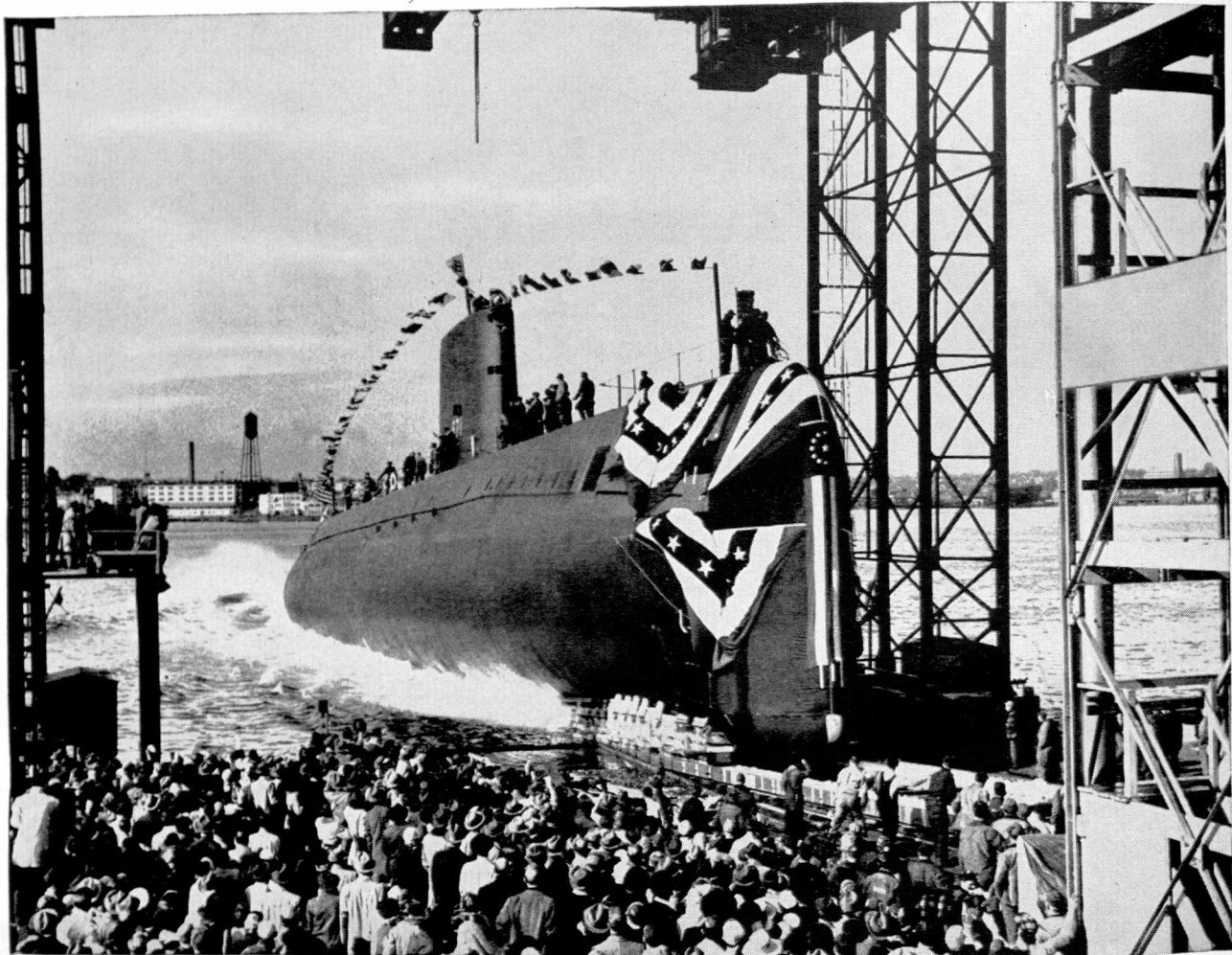
SLIDING DOWN THE WAYS at Groton, Conn., goes the USS Nautilus, newest and fastest member of our undersea fleet. During welding, Worthington heavy-duty turning rolls rotated the hull sections.
