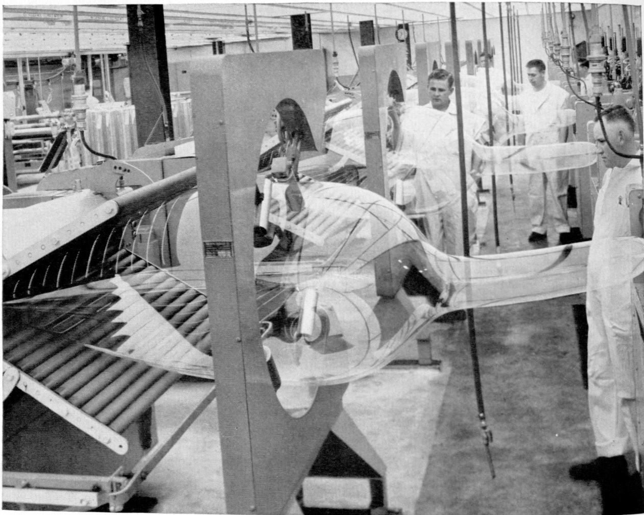
Saran Wrap is stretched by injecting compressed air to form a bubble \frac{1}{2} mil in thickness which is then compressed and wound.
