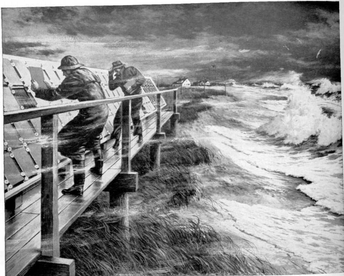
Ocean Laboratory —here at its big Kure Beach, N. C., Testing Station, Inco exposes thousands of metal specimens to the corrosive effects of salt spray, salt air, salt water.
