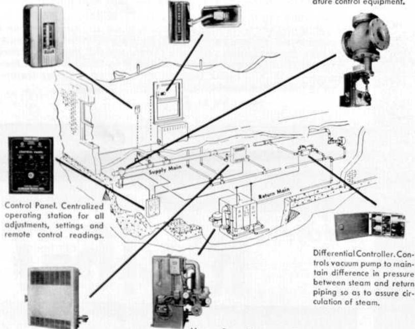
Control Panel. Centralized operating station for all adjustments, settings and remote control readings.
