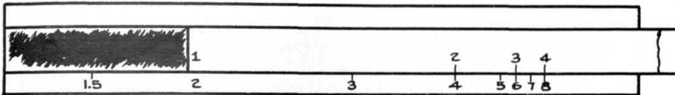
The slide rule above multiplies  $2 \times 4$  for the answer 8. Vertical lines on both scales represent the logarithmic values of numbers but are marked by the numbers themselves. In this way transition of a number to or from its logarithm is done without notation of the logarithm itself.
