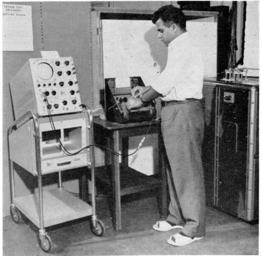
Just inside the front door is a small Sonntag fatigue machine. A strain gage is mounted on the fatigue specimen, and the gage output is fed to an oscilloscope via the amplifier adjusted by T.V. Kameswara Rao of India.
