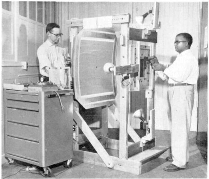
Dr. William A. Bradley and Mr. B. Basava Raju are posing with the apparatus which they built for studying the behavior of plates by an optical interference method.
