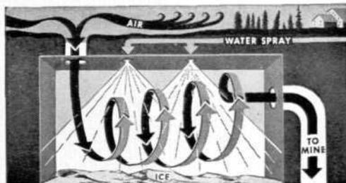
In winter, cold air is blown through sprays of warmer water. The water loses its heat, freezes into mountains of solid ice. In the process, the latent heat of freezing is transferred to the air, warms it up for use inside the mine.
