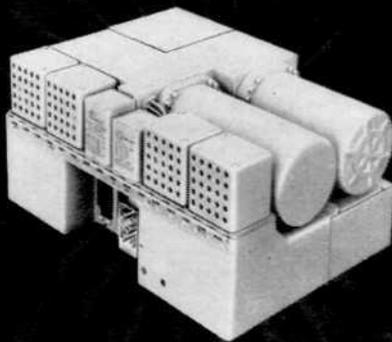
This electronic centralized air data computing system, pioneered by AiResearch engineers, now enables aircraft to operate at maximum efficiency continuously. By sensing air conditions surrounding the airplane, it automatically makes **in-flight** adjustments and feeds vital information to the pilot. This centralized combination of transducers, computers and indicators is **the** most complete air data computing system ever Produced by any manufacturer.
