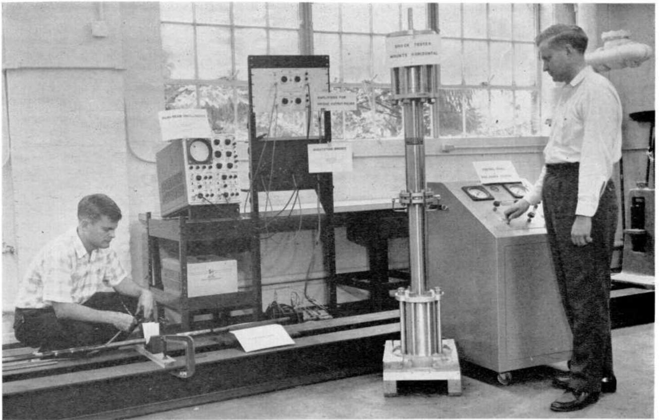
Dr. Lawrence E. Malvern is at the control cabinet of the Hygee shock loader and Ulric Lindholm is checking a connection. Their research is into the propagation of plastic waves.
