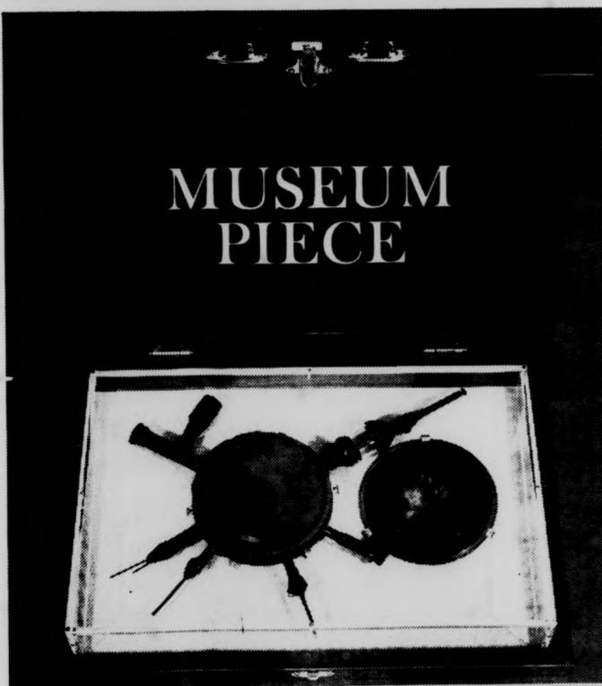
This cyclotron was built and operating by the fall of 1930 and reported at the Washington April Meeting (Phys. Rev. 57, 1707, 1931). The diameter of the chamber was about 5 inches. Placed between the 4-inch diameter poles of a magnet with a field of 12,700 gauss and 2,000 volts on its single disc, it produced 80,000 volt hydrogen molecule ions trapped and measured in a Faraday cage to which a measured and adequate decelerating voltage could be applied.
